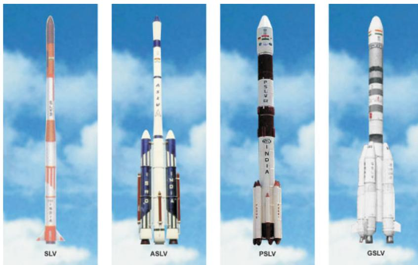
Figure 1.6 Various satellite launch vehicles of ISRO.
