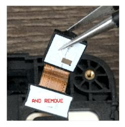
Next we will remove the rear camera. This is basically the same process. Simply unplug the camera from the board and remove. Notice in the photos that you can now see the microphones on the device as well as the light sensor. I prefer to remove these as well.
