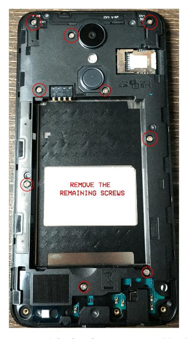
With the antennas removed it is time to remove all of the remaining screws on the back of the device. We are going to begin getting into the actual guts of the device. This is where all the fun is.
