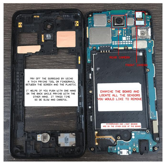
Once all the screws are removed slide a thin prying tool or a fingernail in between the glass of the screen and the plastic surround. Work your way around the device until it pops off completely, exposing the main board. It also helps if you press on the back of the device with the hand holding it while you pry it apart. Take your time with this part or you could ruin the device!
